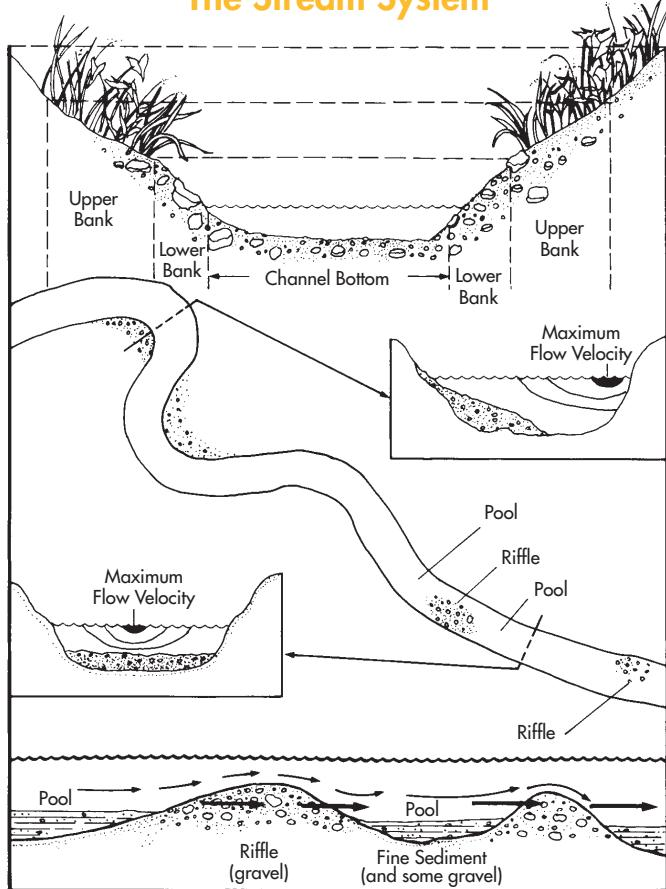
The above diagram shows the water flow and major structures of a stream. Notice how the pools and riffles alternate. A major feature of the riffle is that water flows through the gravel as well as over it. This enables small fish and small benthic invertebrates to obtain the oxygen they need while being protected from predation by larger organisms such as fish.
